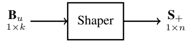
Fig. 3. Shaper maps k uniform bits to n amplitudes. The amplitude sequences are taken from an n -sphere. As n \rightarrow \infty , the distribution of the amplitudes converges to a one-sided Gaussian. Note that each sequence is selected with equal probability. Shaper addresses these sequences with the enumerative algorithm.
