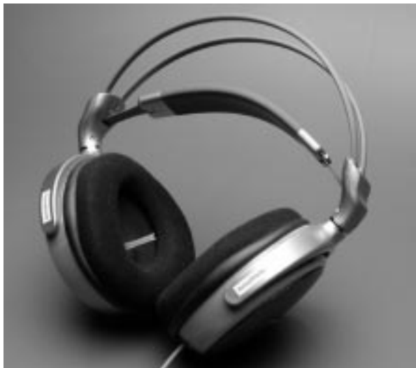
Fig. 4: Headphones with integrated microphones. The silicon tube runs from the microphone to the ear-canal entrance.
