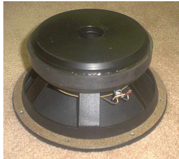
Figure 7. Photograph of the high-BL driver. The device is 26 cm in diameter and the massive magnet structure is 19 cm in diameter.
