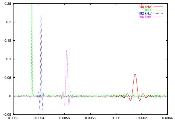
Figure 2: Responses (from left to right) of a DSD, a 192 kHz, a 96 kHz and a 48 kHz system on a -6 dB block input ('click') of 3  $\mu$ s duration, and amplitude 0.25. Note the linear amplitude scale.
