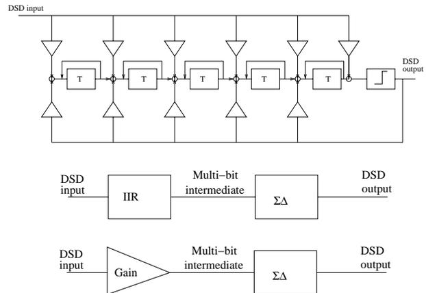
Figure 5: Top: 5th order SDM with IIR filtering. Middle: The equivalent schematic, explicitly including the multi-bit intermediate path. Bottom: A simple example showing multi-bit processing is always necessary; applying gain to a 1-bit signal transforms it into a multi-bit signal.
