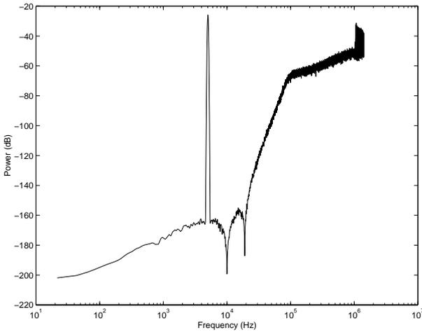
Figure 3: Typical output spectrum of an SDM (5 kHz, -6 dB input).
