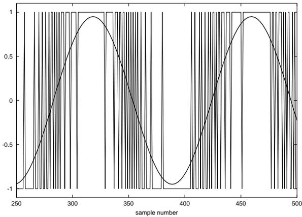
Figure 1: Sine wave in PCM and DSD format. Positive sine wave values result in a large number of +1 values, negative in -1 values.
