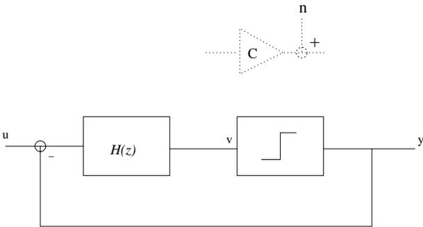
Figure 4: Schematic representation of a feed forward SDM. A linear replacement model for the quantizer is shown dotted.
