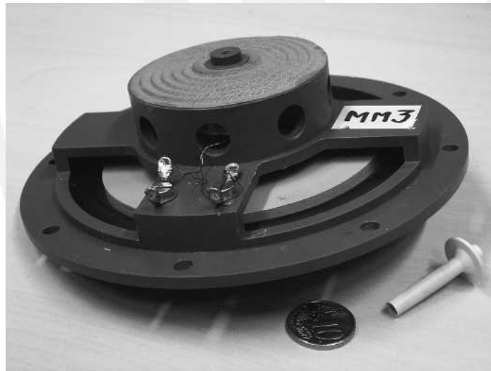
Fig. 8. Prototype driver (MM3c) with a 10 Euro cent coin. At the position where a normal loudspeaker has its heavy and expensive magnet, the prototype driver has an almost empty cavity. Only a small moving magnet is necessary, which is shown at right.
