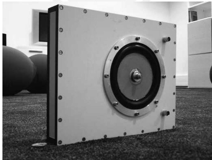
Fig. 9. Prototype bass transducer (MM800) in 1-1 cabinet (1-Euro coin for size comparison, lower left-hand corner) with a resonance frequency of 55 Hz.
