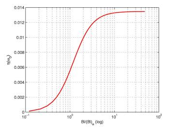
FIG. 4. (Color online) The power efficiency  $\eta(\omega = \omega_0)$  versus the normalized force factor  $Bl/(Bl)_o$  for the driver MM3c, where  $(Bl)_o$  is the optimal force factor given in Eq. (29), in this present case  $(Bl)_o = 1.19$ . The other parameters are given in Table II.
