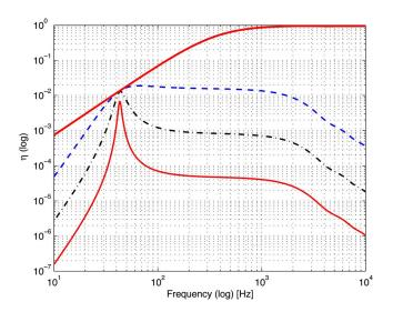
FIG. 3. (Color online) The power efficiency  $\eta$  for the driver MM3c with four *Bl* values: low *Bl*=1.2 (solid), medium *Bl*=5 (dash-dot), high *Bl*=22 N/A (dash), and  $\lim_{B_{l\to\infty}}$  (thick solid), while all other parameters are kept the same as given in Table II. Note that the efficiency is strongly dependent on *Bl* at all frequencies except at resonance, where the efficiency is affected only modestly by *Bl*.
