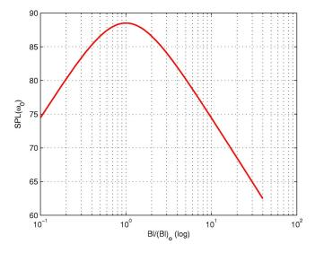
FIG. 2. (Color online) The SPL at the resonance frequency versus the normalized force factor  $Bl/(Bl)_o$  for the driver MM3c, where  $(Bl)_o$  is the optimal force factor given in Eq. (29), in this present case  $(Bl)_o = 1.19$ . The other parameters are given in Table II.
