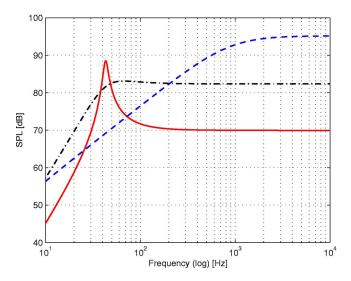
FIG. 1. (Color online) Sound-pressure level (SPL) for the driver MM3c with three *Bl* values: low *Bl*=1.2 (solid), medium *Bl*=5 (dash-dot), and high Bl=22 N/A (dash), while all other parameters are kept the same as given in Table II, all with 1-W input power and at 1 m distance. At the resonance frequency, the highest SPL is obtained by the low-*Bl* driver, while the high-*Bl* driver has at low frequencies—in particular at the resonance frequency—a poor response.
