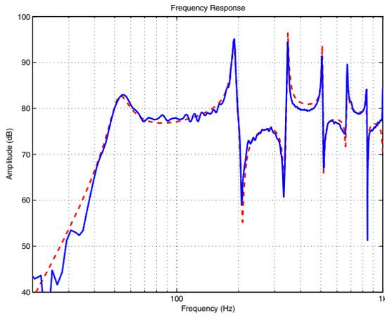
Fig. 16: Measured and calculated frequency response of the system as shown in Figs. 3-b. The port damping in the calculation was  $R_p = 0.01575$  Ns/m. Solid-blue curve: measurement, dashed-red curve: calculation.
