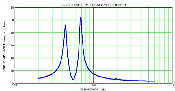
Fig. 8: Electric input impedance (magnitude) as a function of frequency. The parameters are according to Table 1, except for  $m_1$  which has been increased to 24 g in order to obtain  $f_0 = f_b = 55$  Hz,  $Bl$  has the theoretical optimal value of  $Bl_o = 11.7$ , and  $V_0 = 2$  l.
