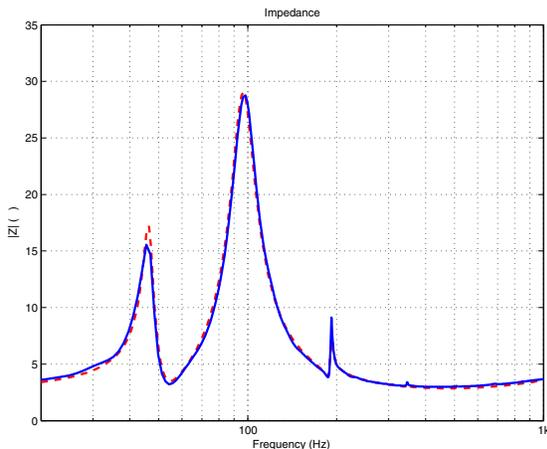
Fig. 17: Measured and calculated electric impedance of the system as shown in Figs. 3-b. The port damping in the calculation was  $R_p = 0.01575$  Ns/m. Solid-blue curve: measurement, dashed-red curve: calculation.
