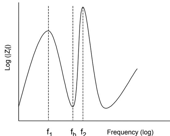
Fig. 4: The impedance of the driver mounted in a pipe. The relevant frequencies are the resonance frequencies  $f_1$  and  $f_2$ , and the Helmholtz frequency or anti-resonance frequency  $f_b$ .
