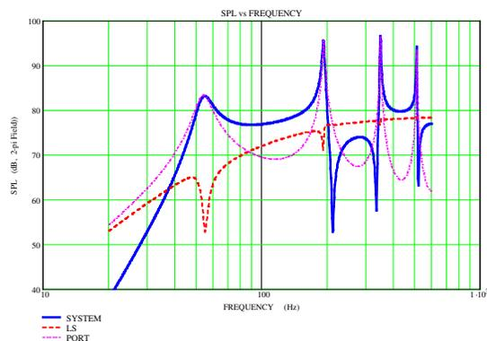
Fig. 12: SPL as a function of frequency for the bass reflex enclosure of Fig. 3-b, where  $f_0 \neq f_b$ ,  $f_0 = f_s = 84$  Hz. System: solid-thick-blue curve. Same loudspeaker: medium-thick dashed red curve. Port only: thin-dashed magenta curve. The parameters are according to Table 1.
