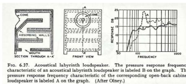
FIG. 6.37. Acoustical labyrinth loudspeaker. The pressure response frequency characteristic of an acoustical labyrinth loudspeaker is labeled B on the graph. The pressure response frequency characteristic of the corresponding open-back cabinet loudspeaker is labeled A on the graph. (After Olney.)
