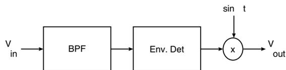
Fig. 15: Set-up of the mapping scheme. The boxes labeled ‘BPF’ and ‘Env. Det.’ are a band-pass filter and envelope detector, respectively. The sinusoid has a fixed frequency equal to  $f_{work}$ . The signal  $V_{out}$  is fed to the power amplifier and finally to the driver.
