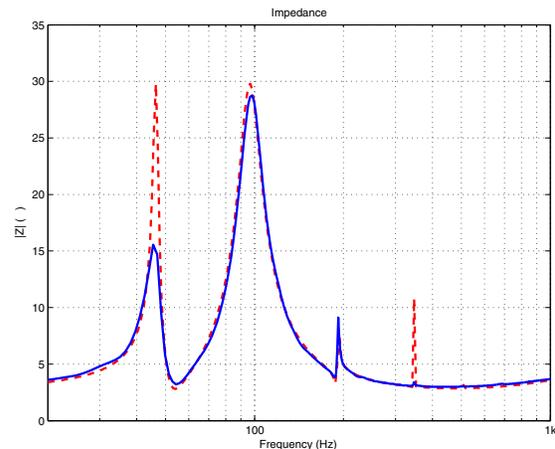
Fig. 19: Measured and calculated electric impedance of the system as shown in Fig. 3-b. The port damping was almost neglected in the calculation. Solid-blue curve: measurement, dashed-red curve: calculation.
