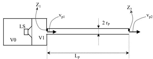
Fig. 5: The mechanical impedances  $Z_1$  and  $Z_2$ , and velocities  $v_{p1}$  and  $v_{p2}$  in the system's pipe.
