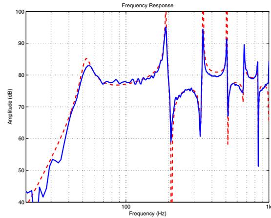
Fig. 18: Measured and calculated frequency response of the system as shown in Figs. 3-b. The port damping was almost neglected in the calculation. Solid-blue curve: measurement, dashed-red curve: calculation.
