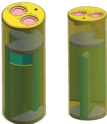
Fig. 14: Drawing of the the experimental set-up. The opening at the front of the pipe in the left drawing is the ‘end of the pipe’. The cavity between the drivers and the grey upper disc is volume  $V_1$ .
