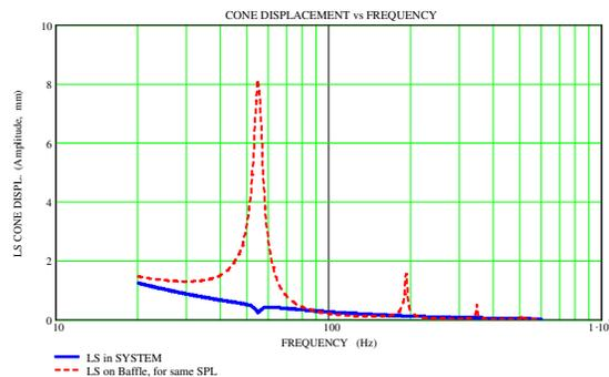
Fig. 9: Cone displacement as a function of frequency. Loudspeaker in system: solid-thick-blue curve. Same loudspeaker in an infinite baffle with the same SPL as the band-pass box: dashed red curve. The parameters are according to Table 1, except for  $m_1$  which has been increased to 24 g in order to obtain  $f_0 = f_b = 55$  Hz,  $Bl$  has the theoretical optimal value of  $Bl_o = 11.7$ , and  $V_0 = 2$  l.
