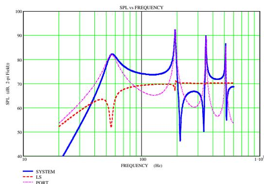
Fig. 10: SPL as a function of frequency for the bass reflex enclosure as Fig. 3-b. System: solid-thick-blue curve. Loudspeaker: medium-thick dashed red curve. Port only: thin-dashed magenta curve. The parameters are according to Table 1, except  $m_1 = 20.4$  g in order to obtain  $f_0 = f_b = 55$  Hz.
