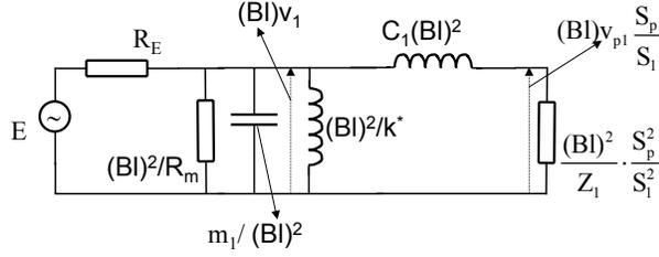
Fig. 6: The mobility-type lumped-element model of the system according to Fig. 5,  $v_1$  is the cone velocity, other parameters are in Table 1.
