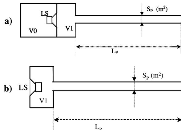
Fig. 3: Schematic construction of the loudspeaker. a) Upper panel: band-pass enclosure with long port. b) Lower panel: bass-reflex enclosure with long port.
