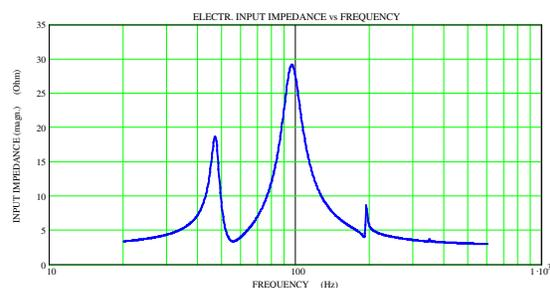
Fig. 13: Electric input impedance (magnitude) as a function of frequency corresponding to Fig. 12, where  $f_0 \neq f_b$ ,  $f_0 = f_s = 84$  Hz.
