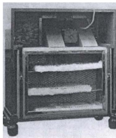
FIG. 1. Acoustical labyrinth with back removed.
