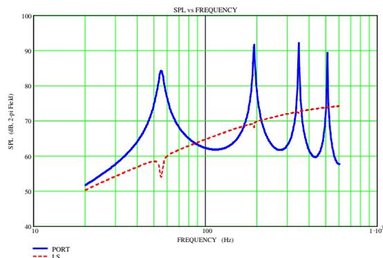
Fig. 7: SPL as a function of frequency. Port-only: solid-thick-blue curve. Same loudspeaker in an infinite baffle with the same excursion as the band-pass box: dashed red curve. The parameters are according to Table 1, except for  $m_1$  which has been increased to 24 g in order to obtain  $f_0 = f_b = 55$  Hz,  $Bl$  has the theoretical optimal value of  $Bl_o = 11.7$ , and  $V_0 = 2$  l.
