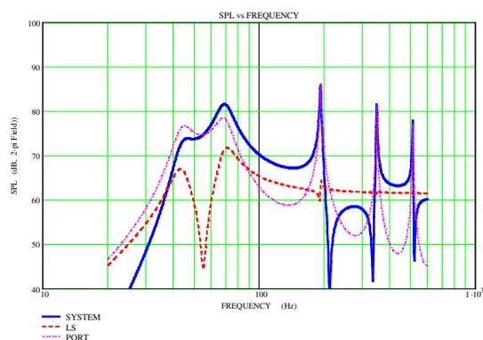
Fig. 11: SPL as a function of frequency for the bass reflex enclosure of Fig. 3-b with a non-optimal  $Bl$ -value. System: solid-thick-blue curve. Same loudspeaker: medium-thick dashed red curve. Port only: thin-dashed magenta curve. The parameters are according to Table 1, except  $m_1 = 20.4$  g and  $Bl = 2$ , which is a factor 0.17 smaller than the optimal value  $Bl_o = 11.7$ .
