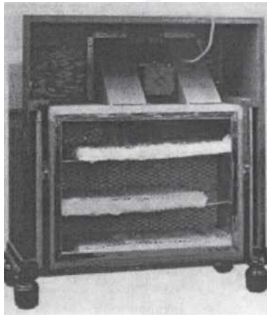
Fig. 1. Olney's acoustic labyrinth loudspeaker [7].
