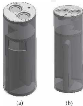
Fig. 14. Experimental setup. “Pipe” is folded four times. Opening in front of cylinder is “end of pipe.” Cavity between the drivers and grey upper disc is volume V_1 and is connected to “pipe” via circle segment.
