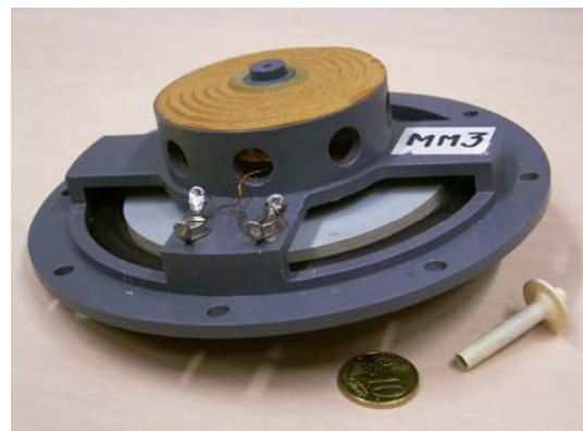
Fig. 3 Picture of the prototype driver (MM3c) with a ten Euro cents coin. At the position where a normal loudspeaker has its heavy and expensive magnet, the prototype driver has an almost empty cavity; only a small moving magnet is necessary which is shown in the right corner.
