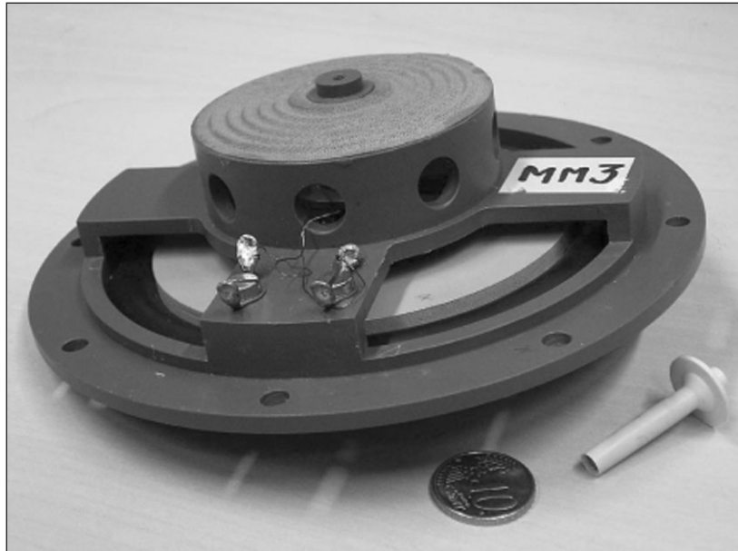
Figure 6 Picture of the prototype low- Bl loudspeaker MM3 with a 10-eurocents coin in the lower middle for comparison purposes. At the position where a normal loudspeaker contains a heavy and expensive magnet, our prototype has an almost empty cavity, because only a small moving magnet is necessary. A copy of this magnet is shown in the lower right-hand corner.
