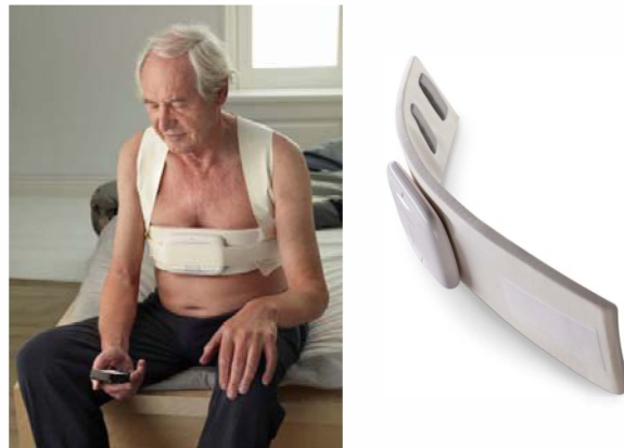
Figure 2. Left: patient performing a trans-thoracic bioimpedance measurement using the BIM at home. Right: the electronics case attached to the textile electrode belt.
