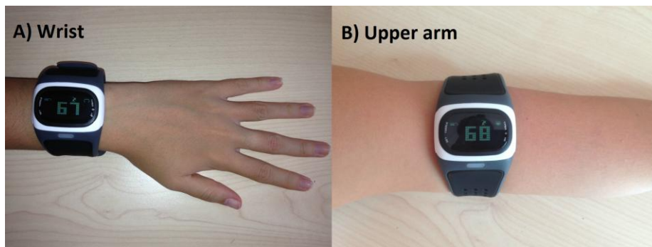
Fig. 2. The MIO ALPHA watch measuring the heart rate, Left, wrist attachment and Right, upper arm.
