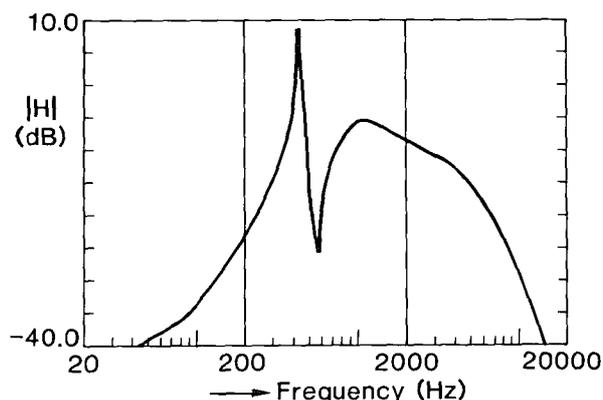
Fig. 4. Amplitude response of transfer function with truncated coefficients.
