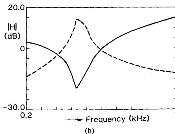
Fig. 2. (a) Amplitude response of two cascaded second-order sections  $H_1$  and  $H_2$ . (b) Amplitude responses of second-order sections  $H_1$  (solid curve) and  $H_2$  (dashed curve).
