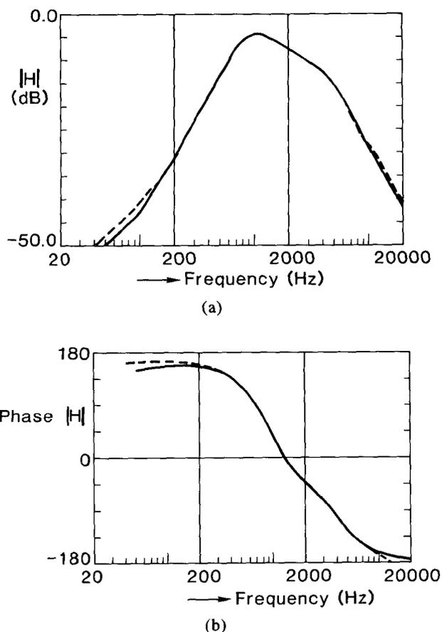
Fig. 3. (a) Amplitude responses. (b) Phase responses. Solid curve—midrange crossover filter loaded with driver (target function); dashed curve— $H(z)$  with truncated coefficients.
